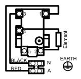
Connect the active and neutral wires to the terminal block and the earth wire to the earth tab (located on the right hand side). Excess wire is not to be looped close to the thermostat or tank.
